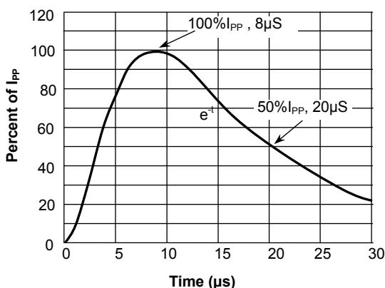
**Fig.4 Pulse Waveform-ESD(IEC61000-4-2)**
